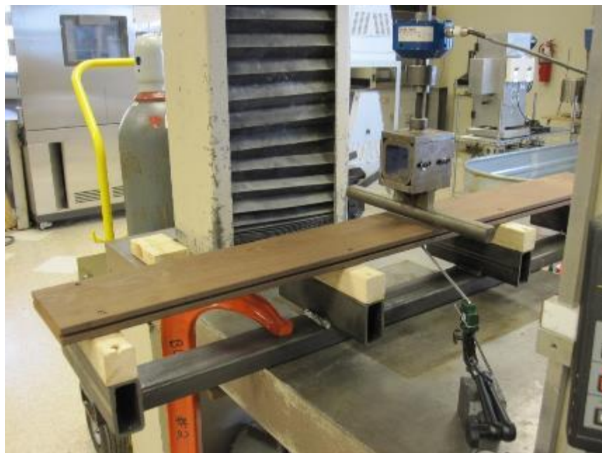
Photo No. 2 Typical Setup for Solid Member Testing
